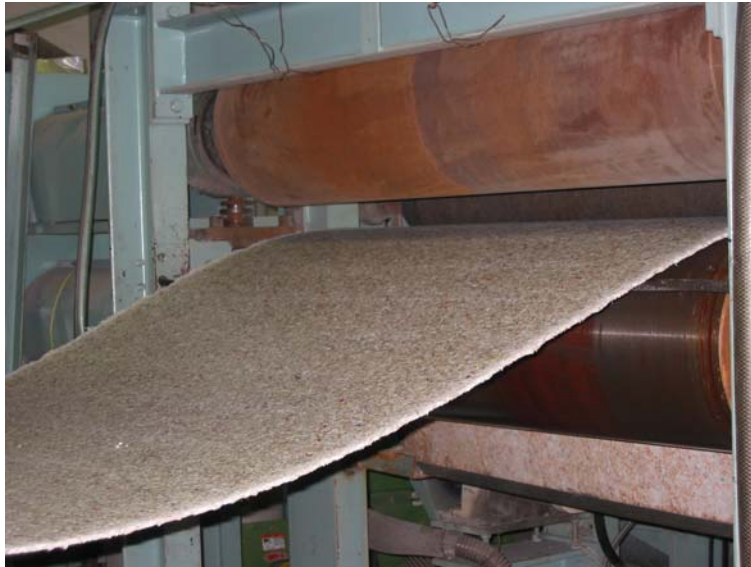
Cooling process after extrusion
